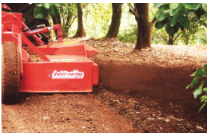
The soil profiler shifts soil from the interrow into the tree row
