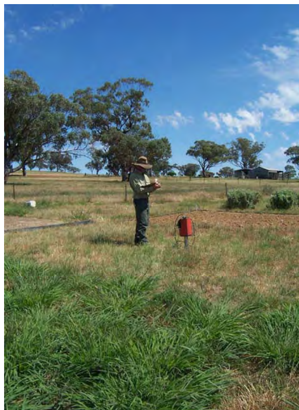
Using a neutron moisture meter to measure stored soil water in a native grass pasture at 'Dunreath', Gowrie, with a Premier digit plot in the foreground.
