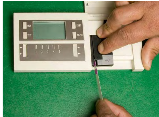
Figure 8. Inserting a test strip into the Merck RQ Flex® meter to take a nitrate reading.
