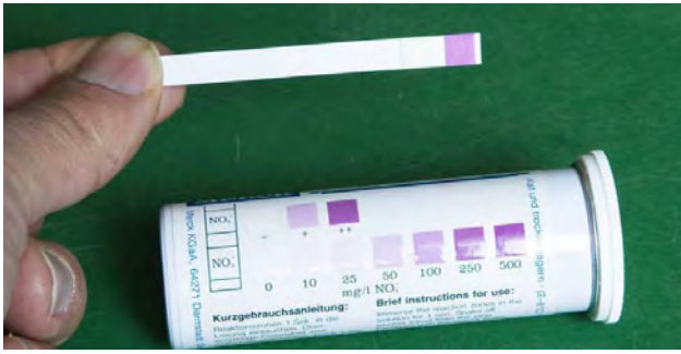
Figure 6. Reading a nitrate result from a test strip using a colour chart.
