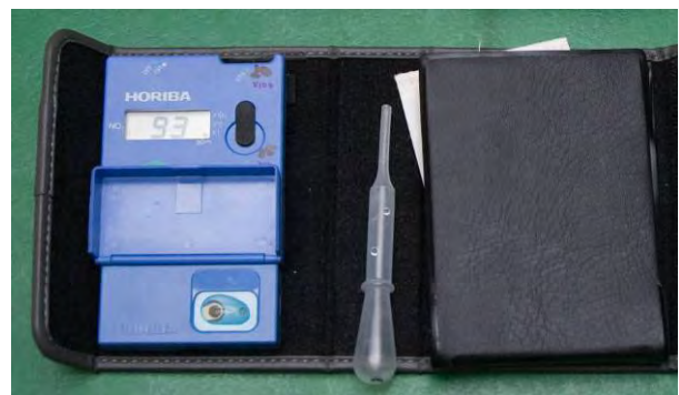
Figure 9. Horiba Cardy® nitrate meter
