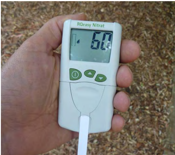
Figure 7. Reading a nitrate result from a test strip using an RQ Easy® meter
