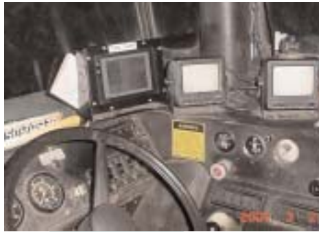
Monitors installed on Pasminco Broken Hill's heavy vehicles to detect light vehicles nearby
