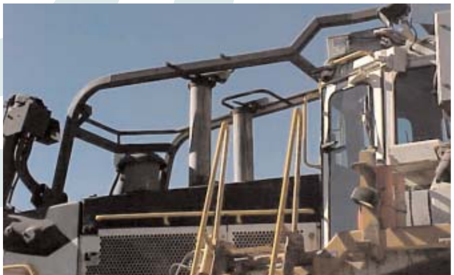
The fall protection frame developed by Mount Thorley Coal Operations personnel
