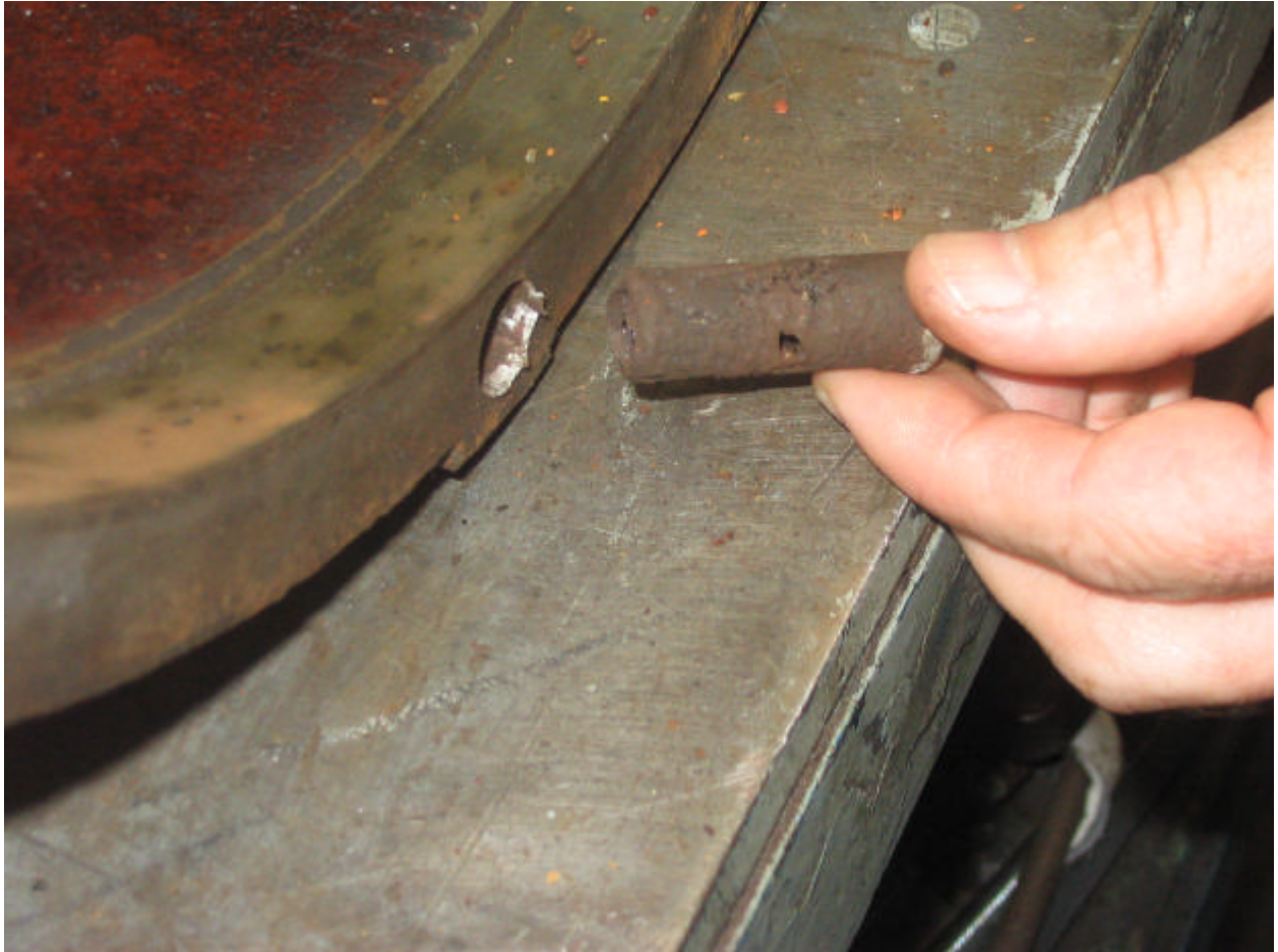
Figure 4. Insert easily removed by hand.
