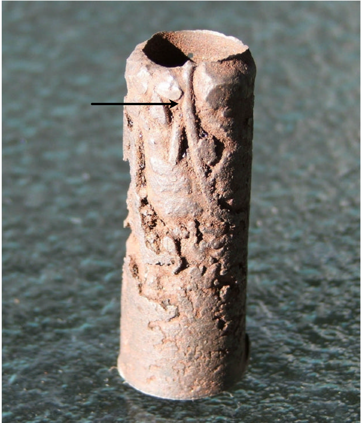
Figure 6. Closer view of insert material after removal from the bolthole (Motor A). Partially melted welding wire is evident.
