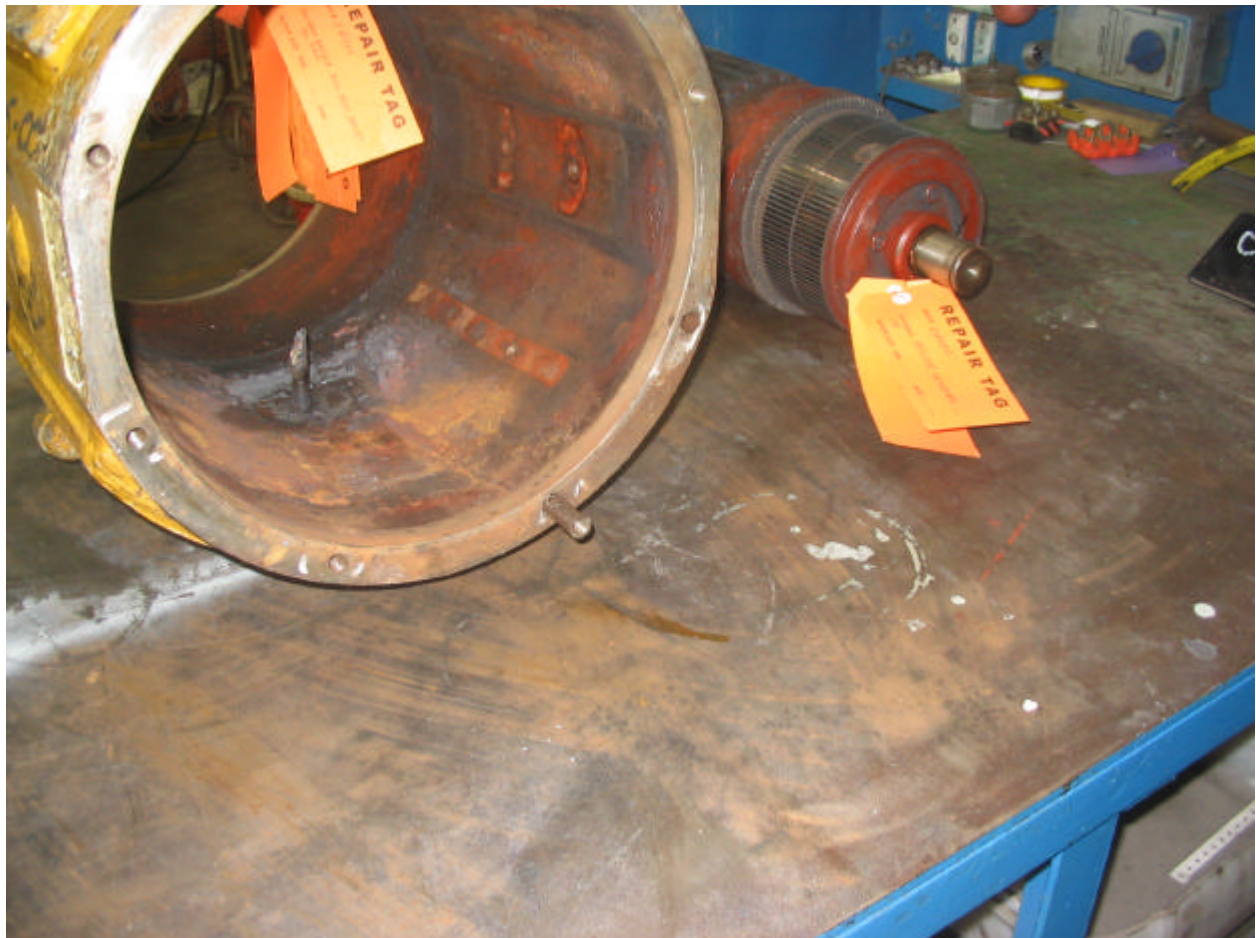
Figure 1. General view of the stator frame end face of Motor A. An insert has been partially removed.
