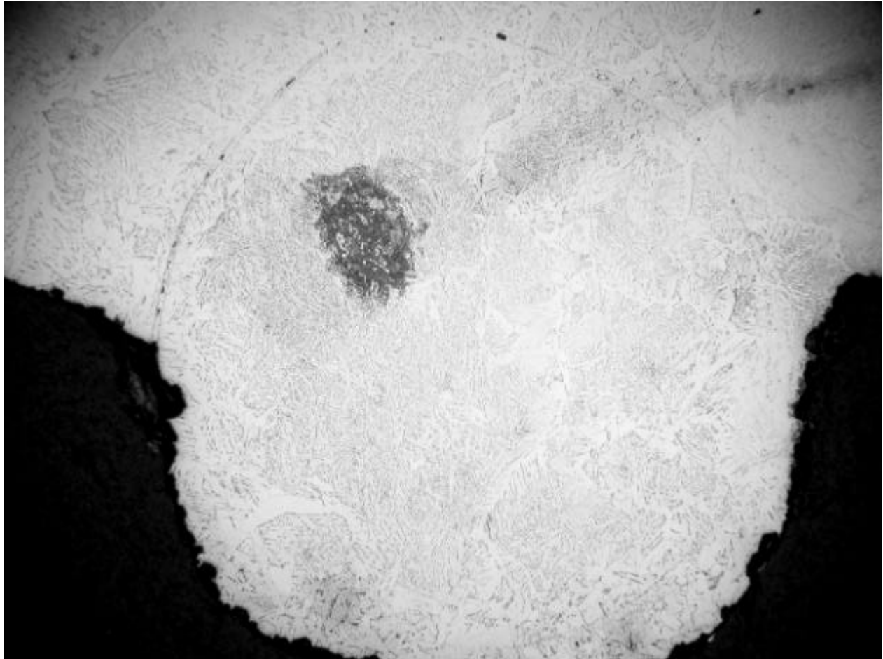
Figure 8. X 100 – 2% Nital etch
