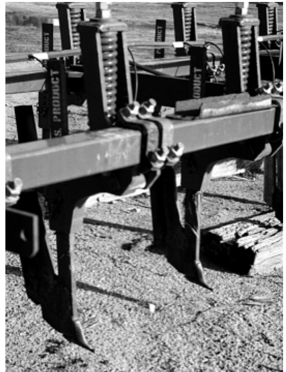
Figure 4 Check tubes & seeding boots of seeders with an undercarriage modified to handle trash.
