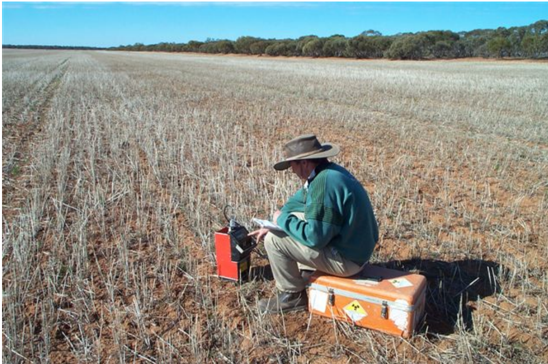
Figure 2 - Measuring stored soil water using a neutron probe.
