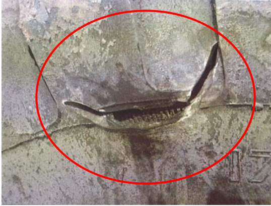
The initial pressure split in the tyre
