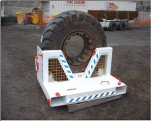
The tyre handler Approximate cost: $7,500 Productivity increased because it takes less time to replace the tyre
