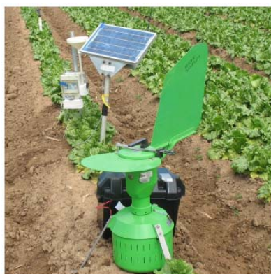
Fig 2 Spore trap and battery (front) and weather station with solar panel (back) located in a lettuce crop.
