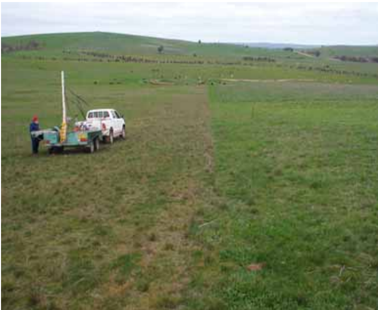
Figure 19. Hydraulic soil corer for obtaining 'intact' soil cores used in the project.
