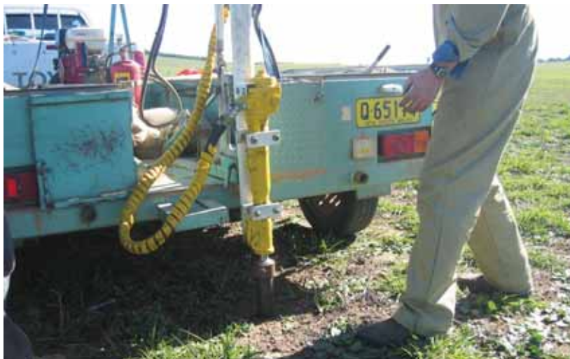
Figure 24. Soil sampling using a hydraulic soil corer.
