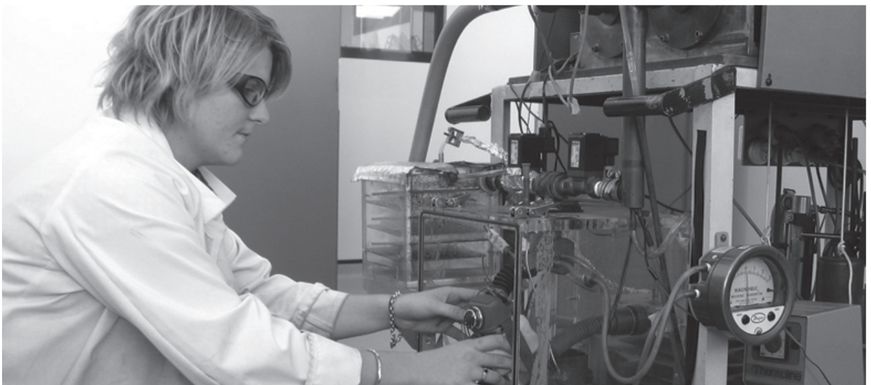
Scientific Officer testing carbon monoxide filter self rescuers for compliance with Australian Standards using lung simulating machines
