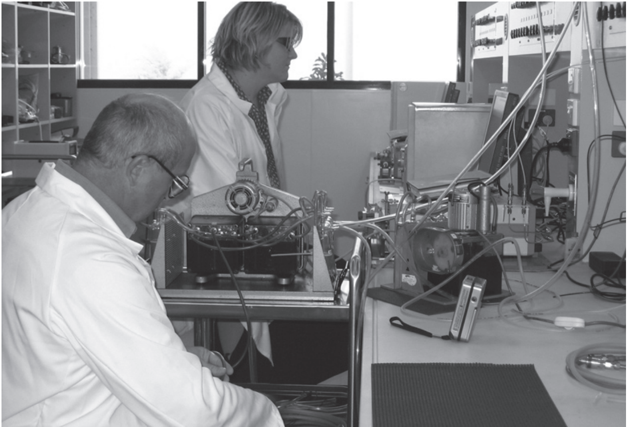
Scientific Officers testing gas samples from underground mines using Wosthoff pumps and Gas chromatography
