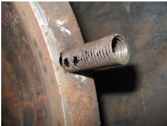
Figures 1 and 2: Two separate examples of the numerous failed thread repairs on a flameproof motor
