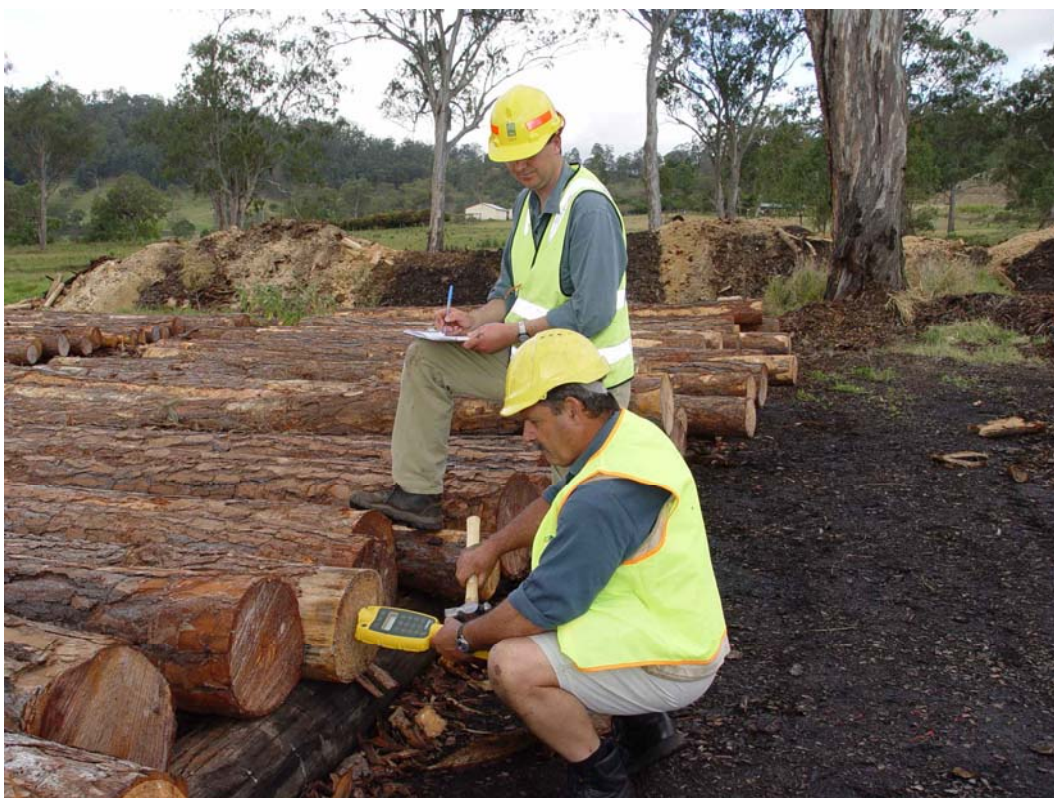
Ross Dickson and Darrel Johnstone using an acoustic tool (Director HM200) to segregate slash pine ( E. elliottii ) logs prior to peeling in an operational study at Norply in Kyogle
