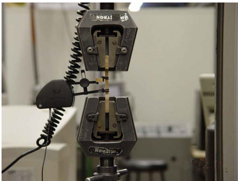
Testing of blackbutt elastic wood properties for incorporation into drying model
