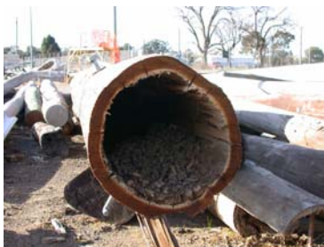
Termite and decay damage to power poles
