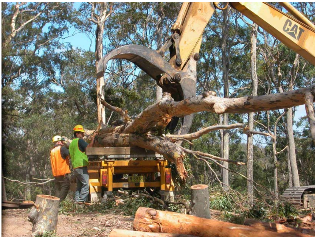
Fabiano Ximenes weighing above-ground biomass on weighing trailer
