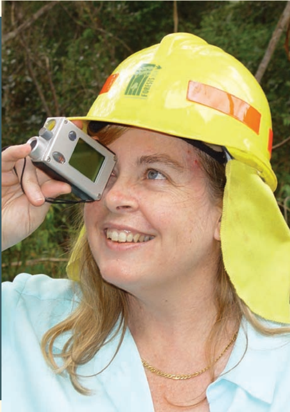
Research Officer – a scientist involved in experimental investigation, data analysis and reporting of specific research projects (picture shows the use of a vertex to assess tree height)
