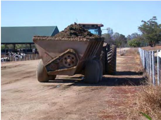
Figure 2. Screened solids from feedlot dairy wastewater being transported for application to an adjacent field.
