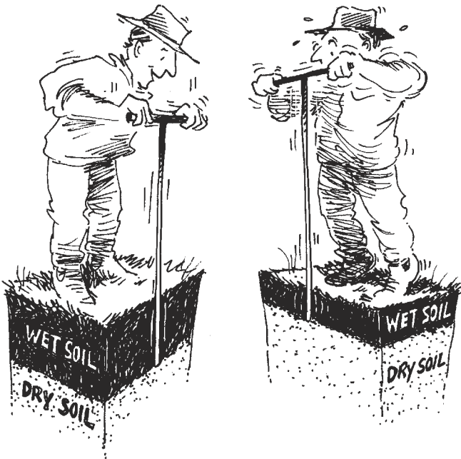
Figure 7. Judging the infiltration depth using a soil moisture probe
