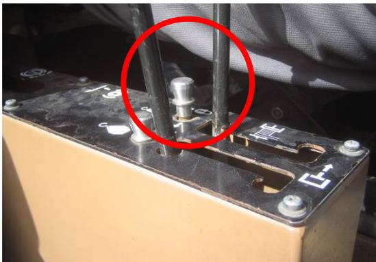
Free fall main and auxiliary hoist controls are not positively interlocked or fail safe.
