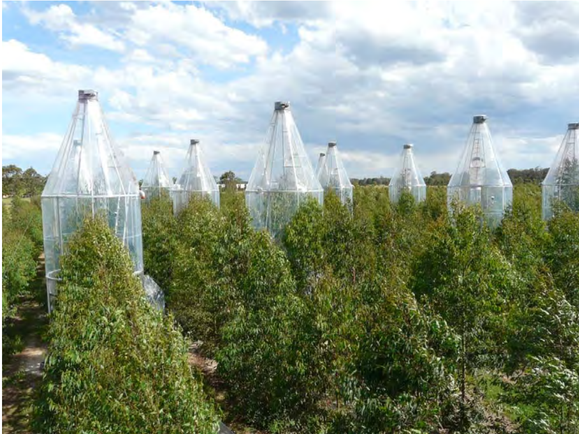
Whole tree chambers (9 m tall) at the field site at the University of Western Sydney's Hawkesbury campus. Photograph by Craig Barton.
