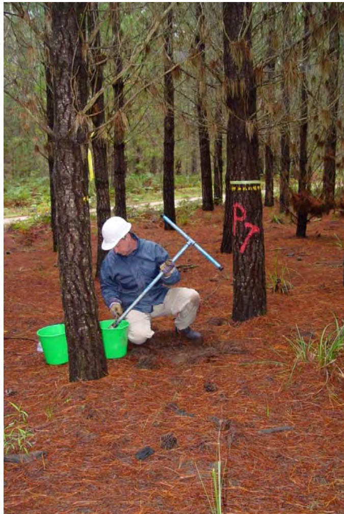
Technical Officer Paul Brooks sampling soil 17 years after biosolids application to determine the long-term soil carbon benefit. Photograph by Georgina Kelly.
