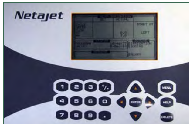
Figure 4. Front panel of a fertigation system control unit that allows setting of water/nutrient mix, electrical conductivity (EC) and pH.
