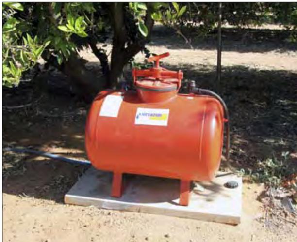
Figure 1. Single fertigation tank in a citrus orchard. This type of equipment is commonly installed down stream of a valve that services a distinct management unit (i.e. block). It generally can only supply a single fertiliser at a time and requires manual operation.
