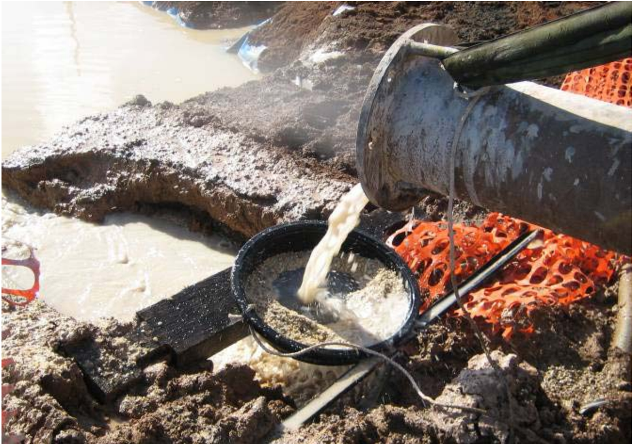
Figure 6 Drilling fluid and drill cuttings exiting the core hole (PEL433 Allambi-1C)
