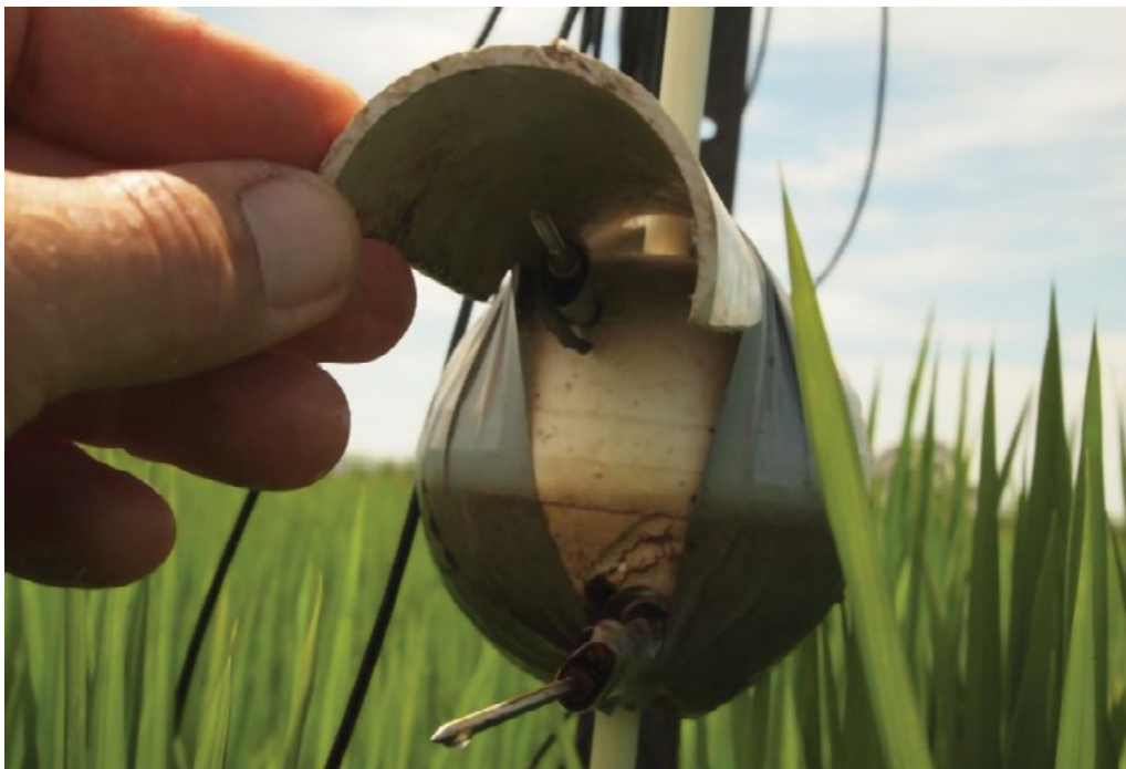
Figure 3. Temperature probes used to measure water and air temperature in the rice crop.
