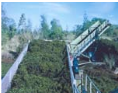
A shore conveyor may be required to get the weed from the harvester to the shore.
