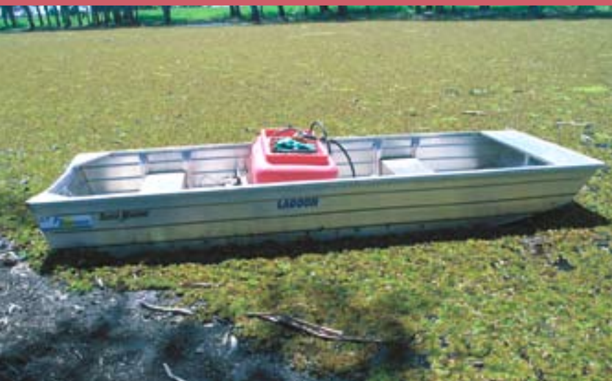
A 200-L spray tank in a flat-bottomed tinny.
