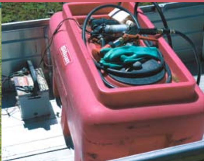
12-volt battery-operated pump for spray tank.
