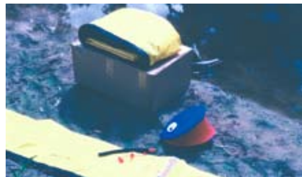
A curtain boom awaiting inflation of the air chamber
