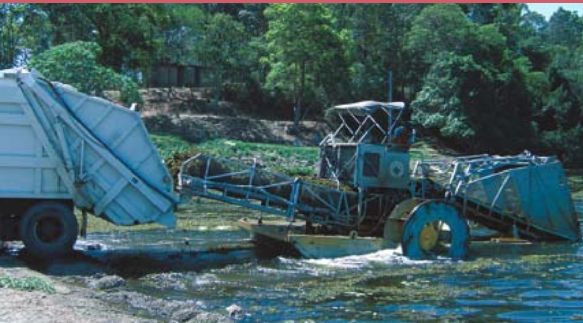
Roy Durrie Russell Rainbird ▲ Mechanical scoop attached to the bow of a 5.25 m aluminium boat. ◀ Harvester unloading salvinia into a compacting garbage truck.
