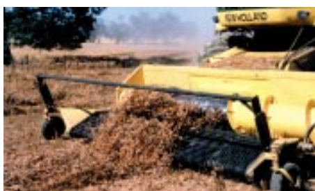
Figure 3 Harvesting narrow-leaved lupins using a pickup front
