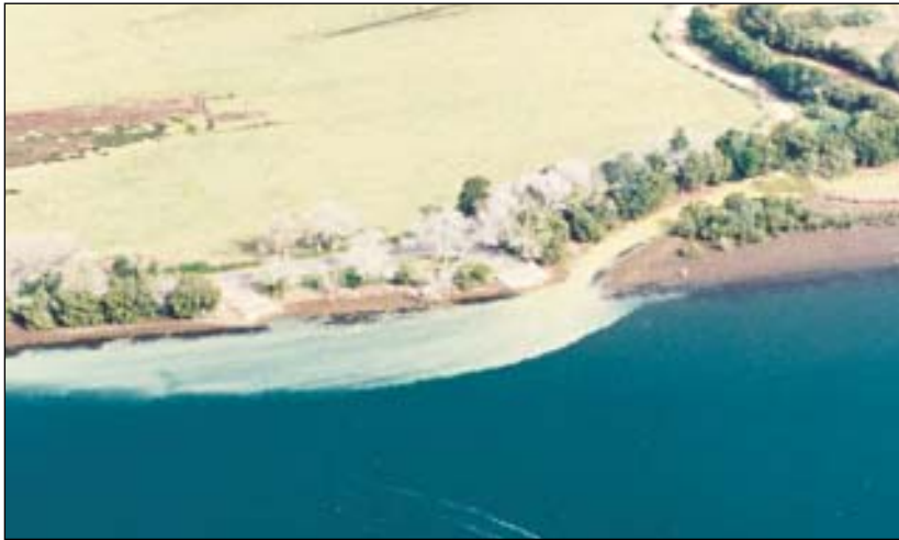
Figure 4. Plume of acidic water entering an estuary – a result of drained acid sulfate soil.
