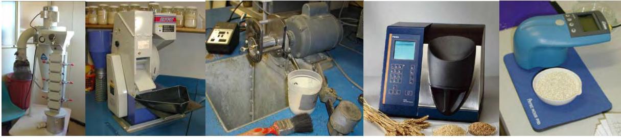
Figure 1. Physical quality assessment. From left to right: aspirator, dehuller, mill, Cervitec and the spectrophotometer.
