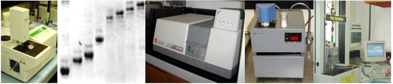
Figure 3. Cooking quality assessment. From left to right: calorimeter, molecular marker, UV-vis spectrometer, viscometer and texture analyser.
