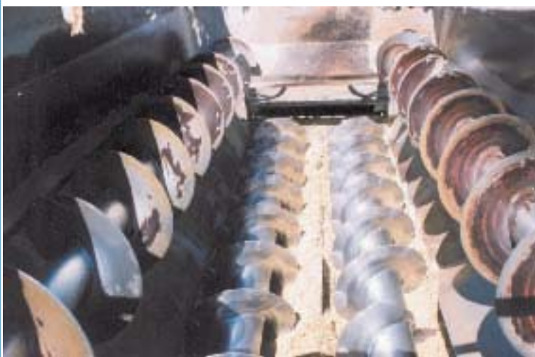
Internal auger system of a mixer wagon.
