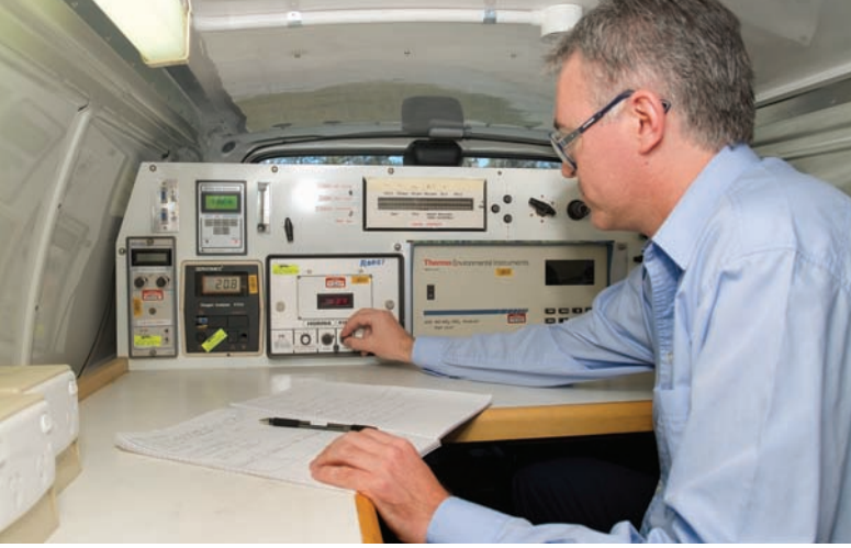
Senior Scientific Officer at the Mine Safety Technology Centre Greg Browning tests gases using the mobile gas testing laboratory.
