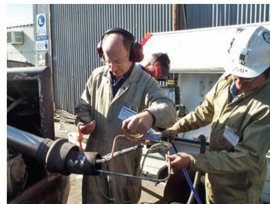
The 2004 Mine Safety Review recommends a stronger focus on mine-related health regulation and monitoring. Diesel particulate emissions are an example of a mine-related health hazard. Photo: NSW DPI, Mine Safety Technology Centre officers test for diesel particulate emissions.
