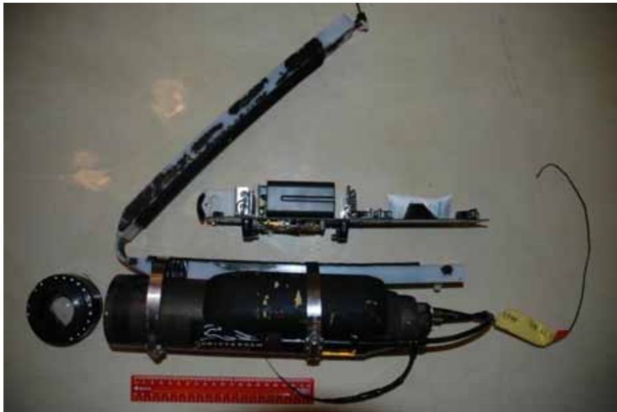
Photo 1. CriterCam electronics including fin clamp and release burn-wire.
