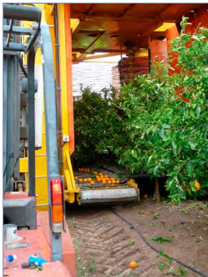
Figure 6. A series of rods gently move through the tree and dislodge the fruit.
