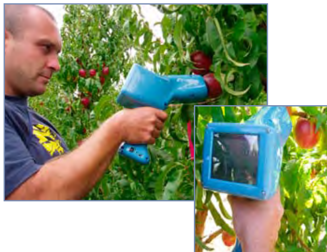
Figure 1. Use of portable non-destructive NIR to measure fruit SSC in the orchard.
