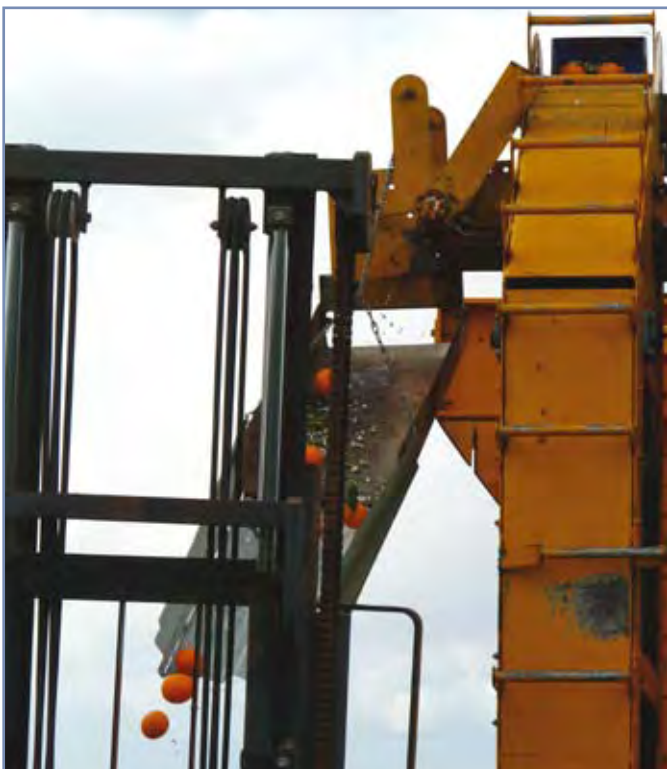
Figure 9. A series of elevators and chutes deliver the fruit to the 5 tonne bin.
