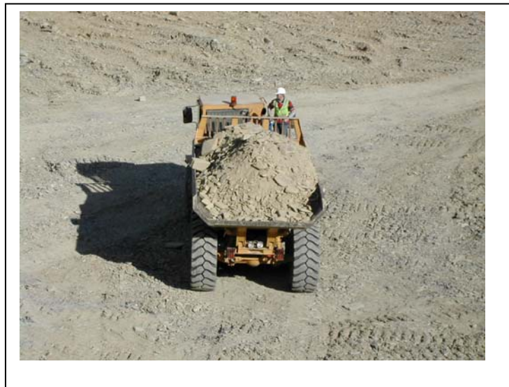
Plate 12.1: Contractor hauling overburden at a slate mine
