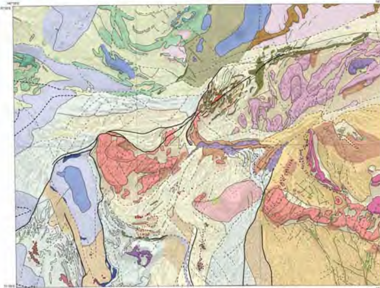
Preliminary version of Geophysical/Geological Interpretation Map for Bourke, overlain on 1VD TMI RTP image
