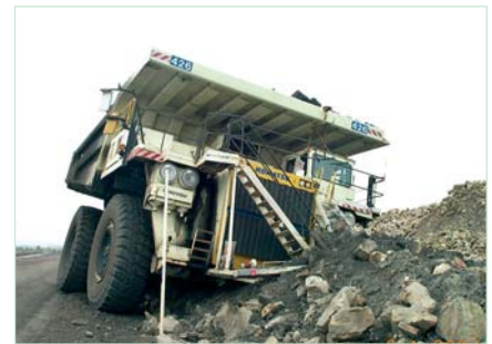
Large Rear Dump Truck run off the haul road due to unplanned movement.
