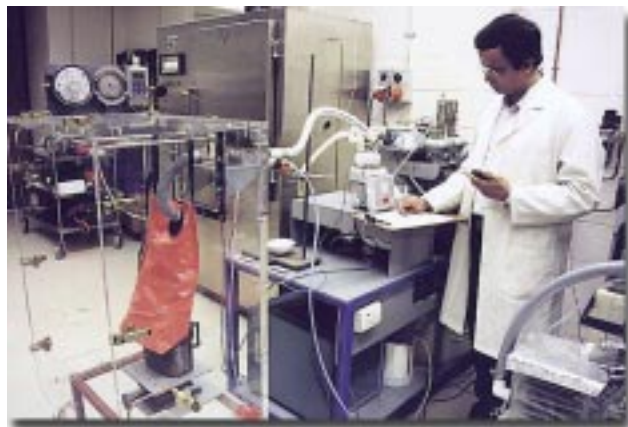
Testing a Fenzy self rescuer on the Department's closed circuit breathing simulator at its Mine Safety Laboratory
