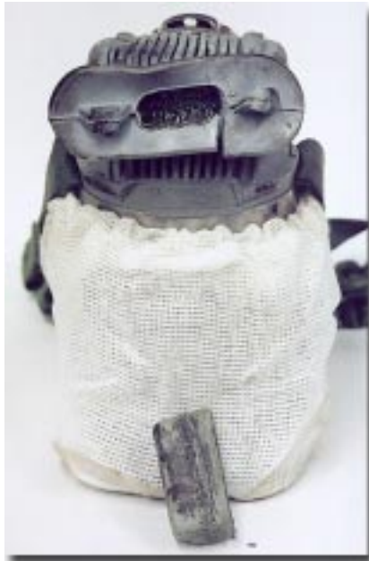
One of the recalled MSA carbon monoxide filter self rescuers showing the poor condition of the mouthpiece
