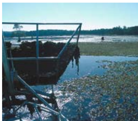
The scoop has a load capacity of 150 kg.
