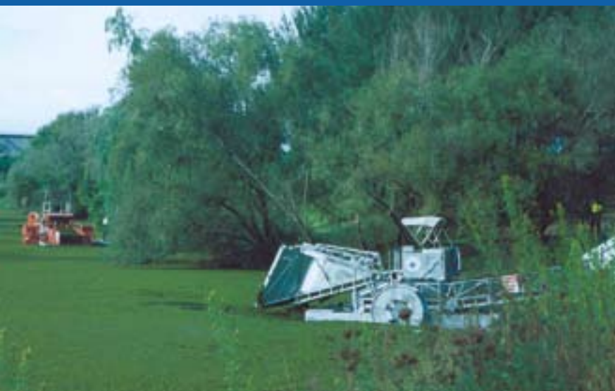
Two 13 m 3 load capacity harvesters were operating on the river for an 8-month period.
