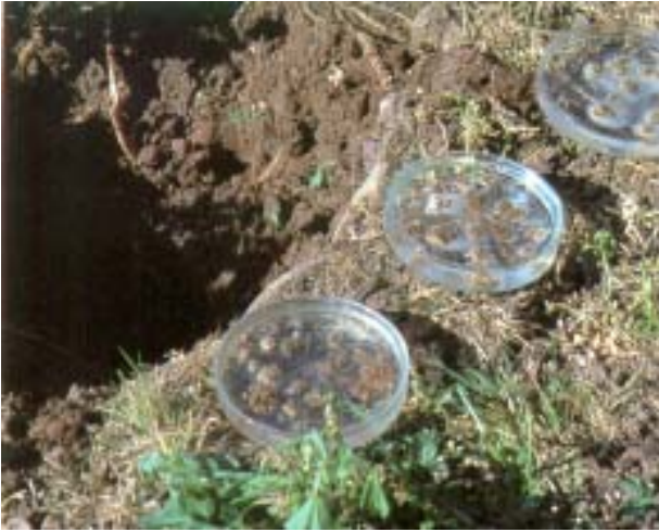
Potential soil structural problems can be identified quickly and easily using slaking and dispersion tests in the field.
