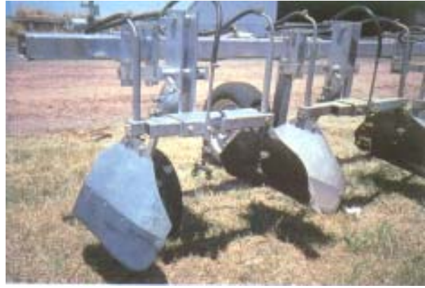
Shielded sprayers can be used for spraying furrows or between plant rows on raised beds.
