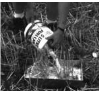
Figure C4-11. Pouring a white paint solution into a soil to assess the presence of continuous vertical macropores.
