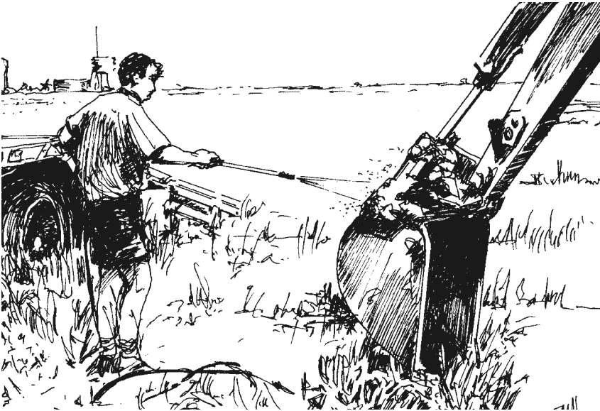
Figure C1-6. Excavation equipment must be disinfected to avoid the spread of cotton disease.
