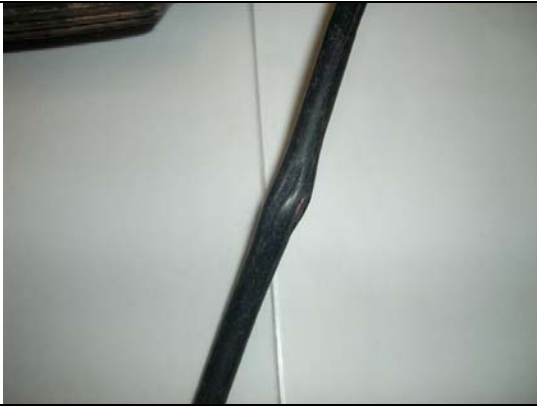
Damaged impact wrench lead
