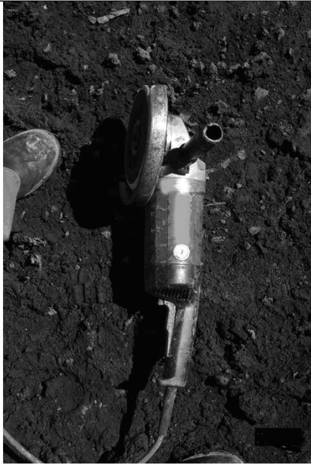
Angle grinder not suitable for the wet and muddy environment
