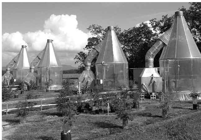
Climate control tree chambers used to investigate climate change impact on tree growth.
