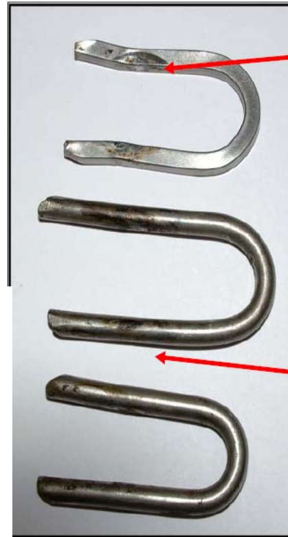
Staples worn and starting to wear where the hose is contacted
