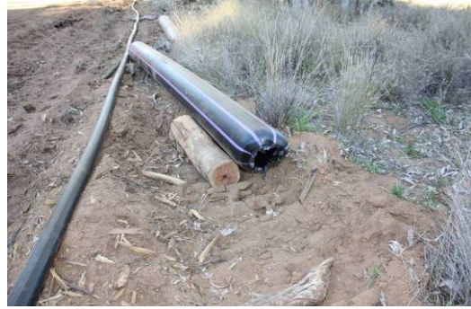
The piece of wood that was placed in the pipe was found at the scene next to a sheared piece of the pipeline.
