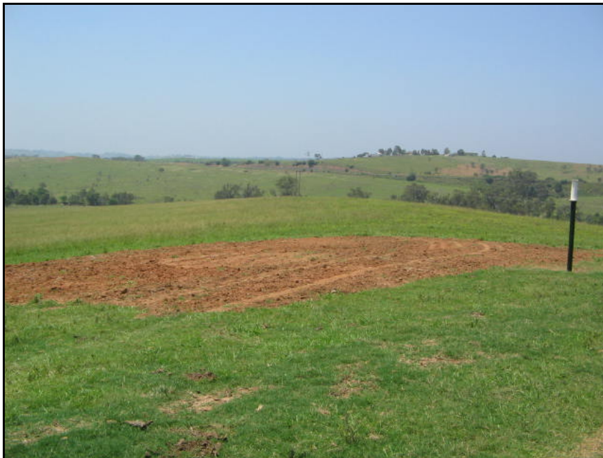
Plate 4: Site rehabilitated with standpipe and Piezometer recorder .Data is sent by telemetry eliminating need to access site.
