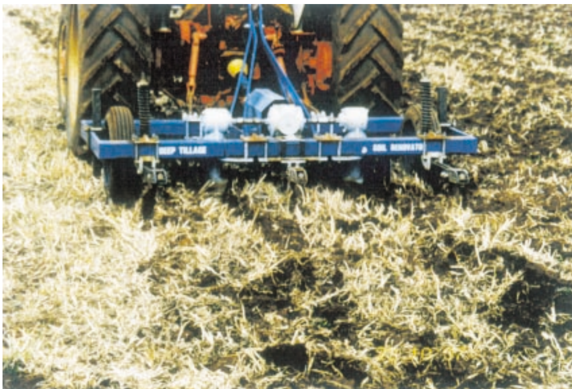
One pass into a sprayed-off paddock is sufficient to prepare a seedbed for planting. Another advantage is that only rows into which potatoes are sown are disturbed by the rotary tines, thereby keeping the area and degree of ground disturbance to minimum. (Guy Van Owen)
