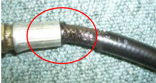
*burst behind the fitting
