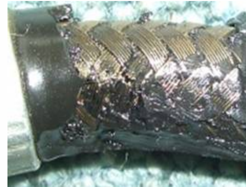
*inner liner cracks at kinked part
