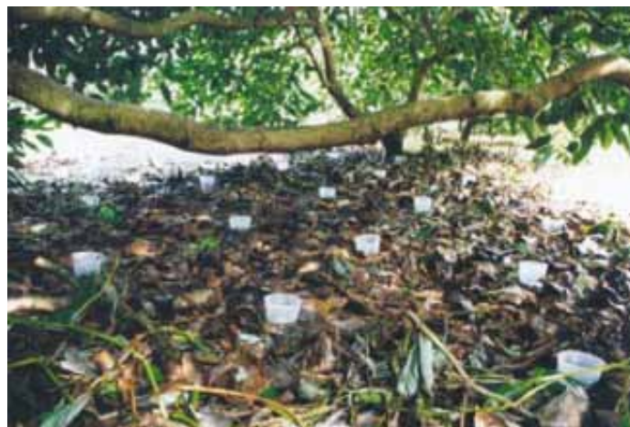
Containers distributed under the trees are used to test for even spread of irrigation flows.
