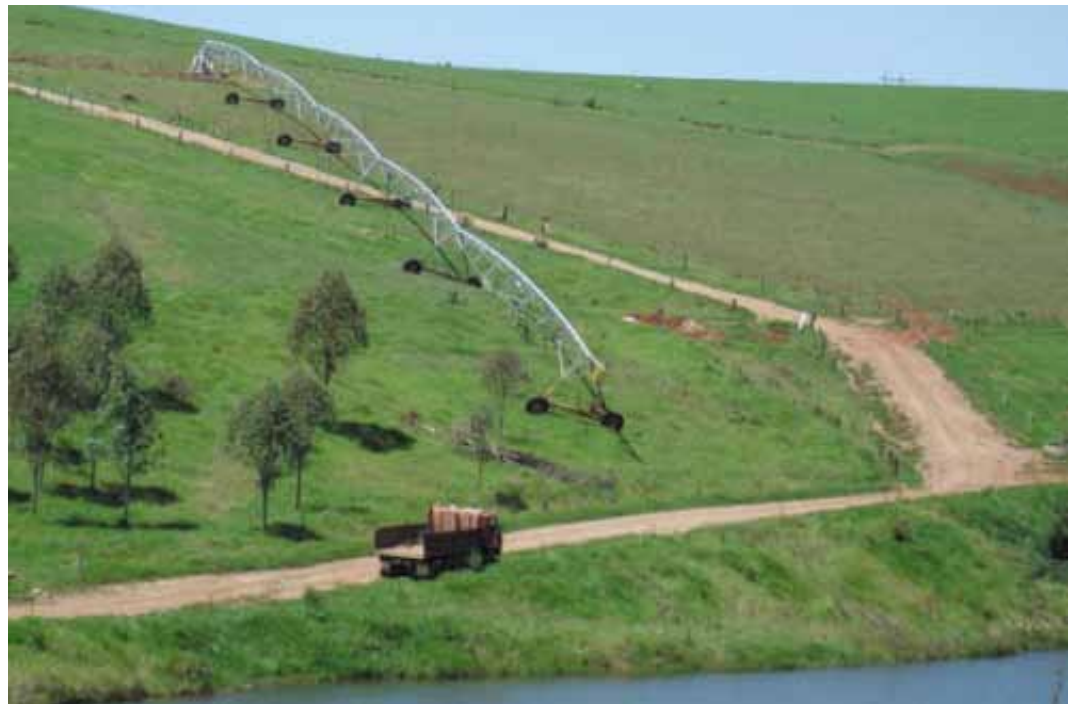
The centre pivot is located on a steep hillside which it handles easily. The track up the hill is too steep for a car. Gates are established in any fences it has to cross.
