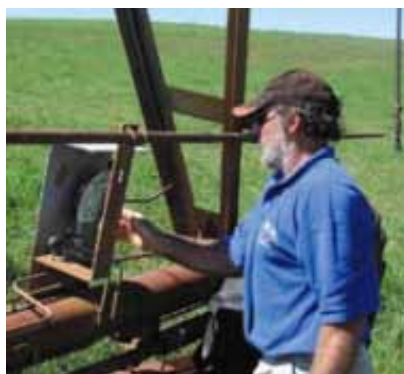
Greg Billings sets the travel speed of the centre pivot. It can apply anything from 5 to 100 mm at each pass.
