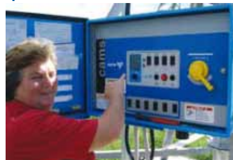
Irene Carle checking the control unit for the centre pivot, allowing for adjustment of water volume.
