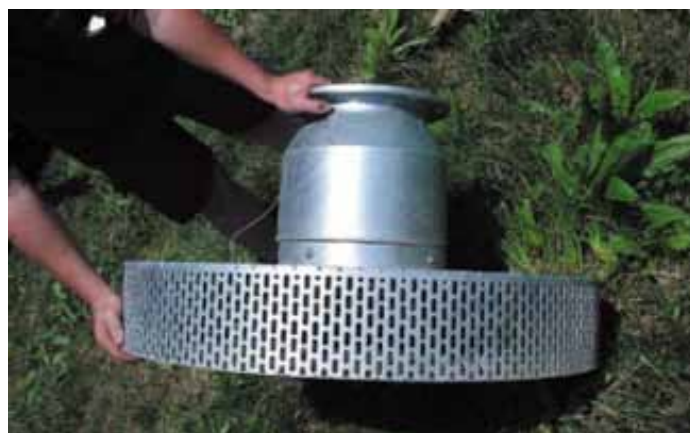
Special foot valve and screen that allows operation in shallow water without sucking air. The device incorporates radial vanes which prevent the inflowing water spinning and developing a vortex.
