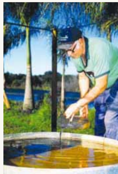
A nursery irrigator measures his daily evaporation to calculate his irrigation requirement. For most purposes, evaporation readings from the Bureau of Meteorology are acceptable.
