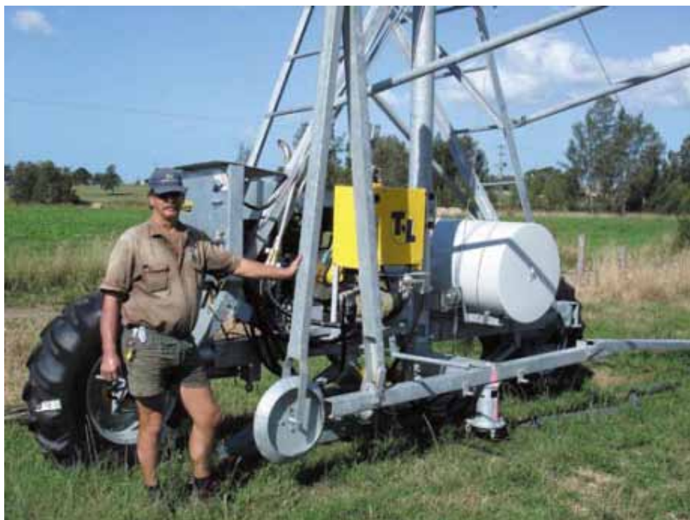
Ric Green with the lateral move irrigator. Beside him is the guide wheel which runs along a furrow cut in the ground to keep the irrigator on line. The control panel behind him allows him to set different irrigation rates as well as control direction of travel. Each tower has its own built in jack which makes swinging the wheels around to allow end towing very easy.
