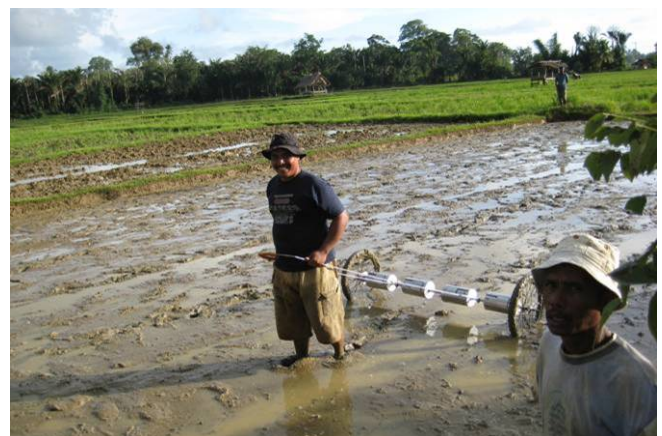
Rice planter in Palembang developed by International Rice Research Institute (left), and model copied by Acehnese farmers and extension staff in Meulaboh using Rizal's son's bike wheels (right). We hope he gets a new bicycle!
