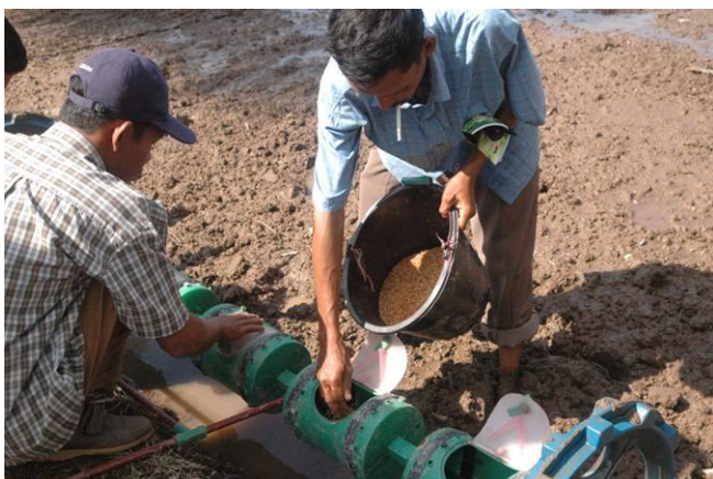
Rice planter in Palembang developed by International Rice Research Institute (left), and model copied by Acehnese farmers and extension staff in Meulaboh using Rizal's son's bike wheels (right). We hope he gets a new bicycle!
