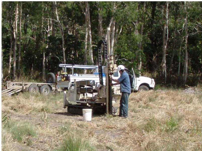
Jeremy Manders working with the Geoprobe coring machine, for a site at Cairns.
