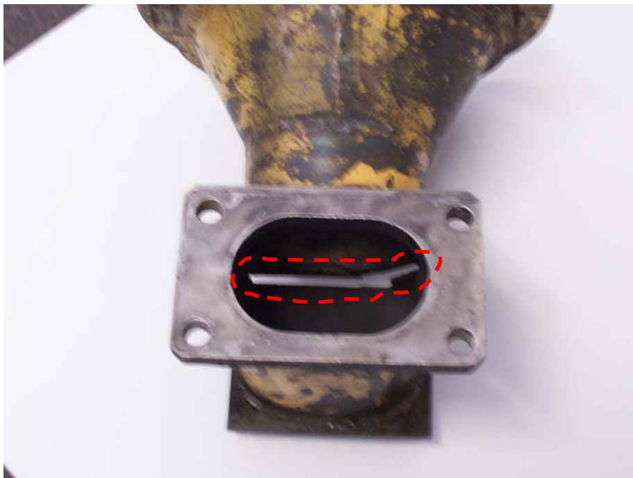
Figure 3 – Photo of cracked manifold. Visible section of crack is circled.
