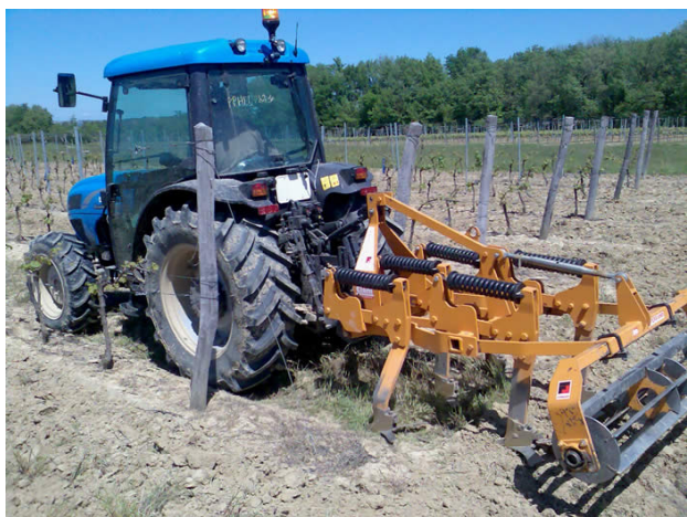
Above: The Actisol two-layer plough. Note the deep tillage tines at the front and the shallow roller cultivator at the rear. Source: www.vignevin-sudouest.com/actions-itv/recherche-itv/images/Actisol3.jpg
