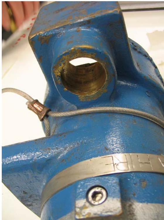
Photo 5. Casing bored to accept a bush – UNACCEPTABLE ARRANGEMENT
