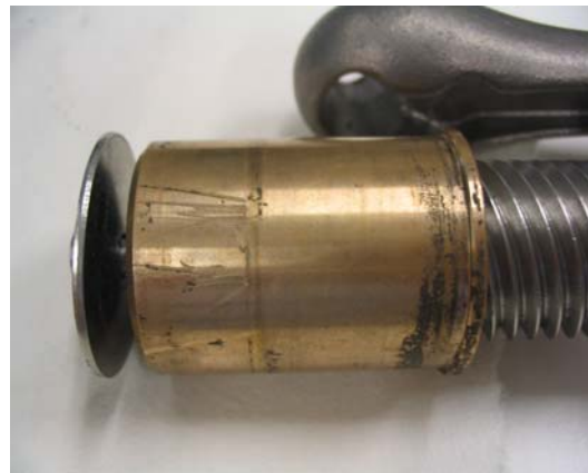
Photo 7. Bush – showing score marks where the grub screw has failed to retain the bush within the receptacle body.
