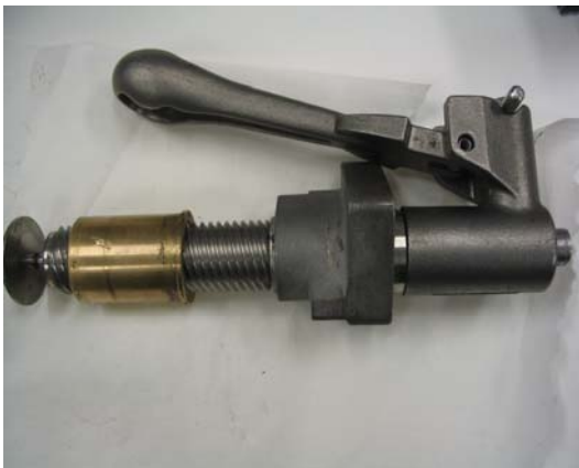
Photo 6. Jacking screw with a threaded bush dislodged from receptacle body – UNACCEPTABLE ARRANGEMENT
